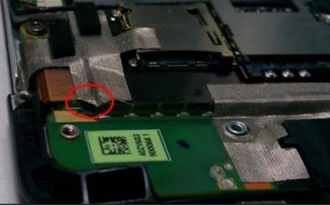
*Inspect and make sure the gasket does not come in contact with the reset pad of the main board.*
