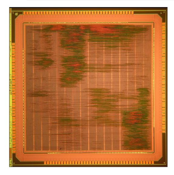
Technology: IHP 0.25µm CMOS Area: ~ 30 mm2 Number of gates: 420,000 NAND Number of pins: 140 signal + 16 power Package: PQFP 208L 28\*28\*3.35P0.5 Peak power: ~1W at 80 MHz, 2.5V Chip testing: Agilent 93000
